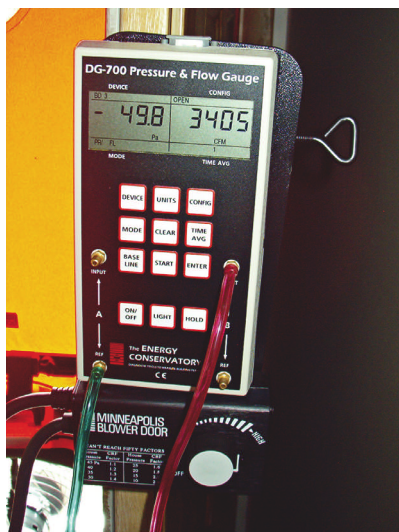
This gauge for the blower door test measures how much the house leaks.
