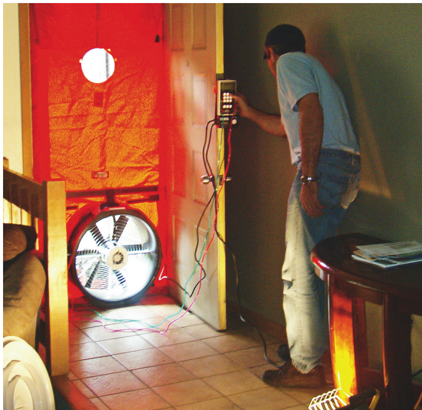
A blower door test reveals air leaks anywhere in the home.
