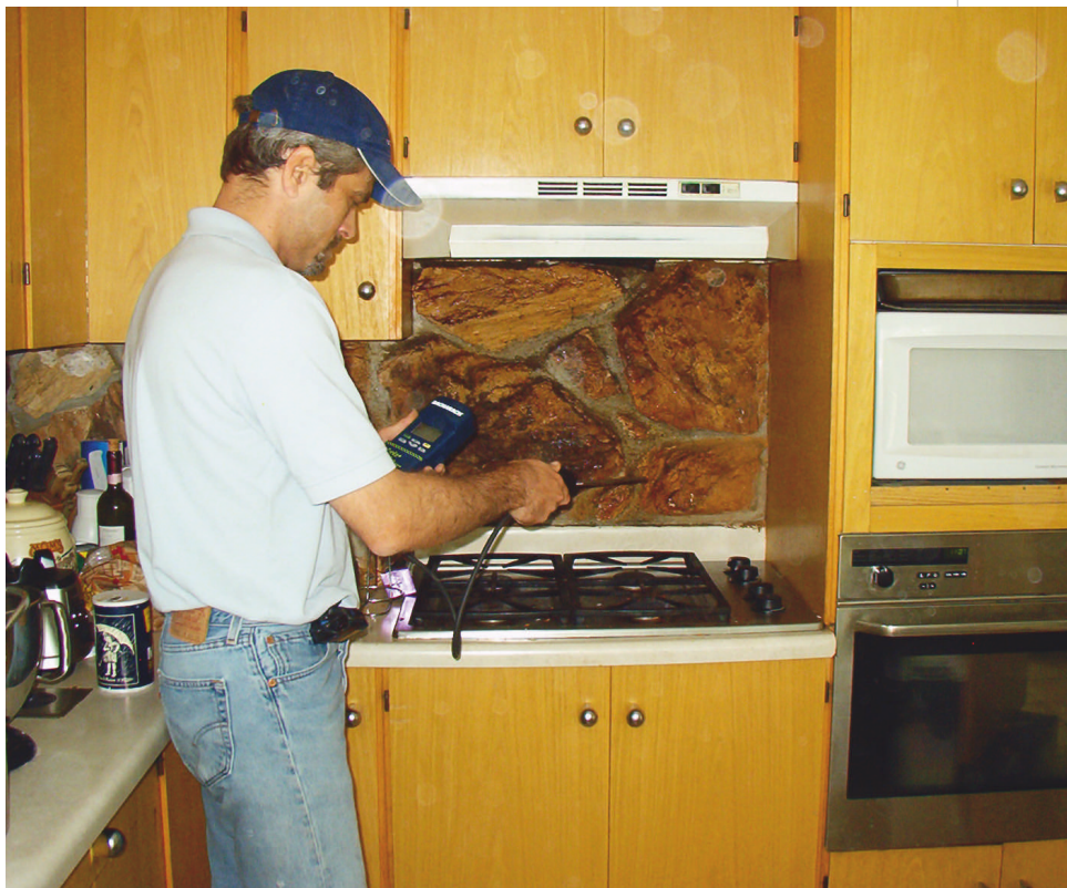
Michael Lotesto tests the air over a lit burner to check the ambient levels of carbon monoxide.
